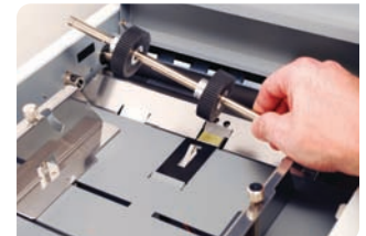
Ensure reliable feeding with easy maintenance feed wheels
